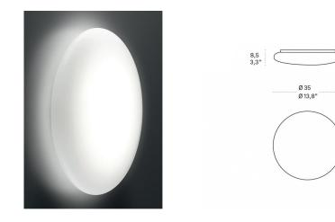
Wall-ceiling lamps with diffuser in mouth-blown, satin-finish opal triplex glass; matt white painted metal frame. The Mentos collection features a special magnet fixing system for the glass component: this system simplifies and speeds up the installation and is highly practical when standard maintenance is required. The product is suitable for indoor use only.
